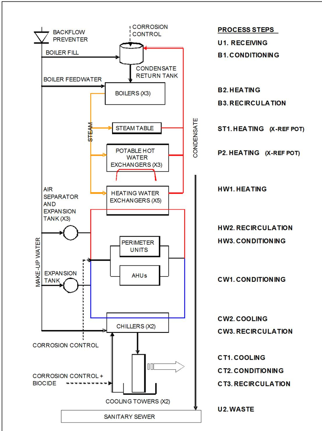
U = utility B = boiler ST = steam table P = primary potable HW = hot water CW = chilled water (evaporator) CT = cooling tower (condensate) X-REF POT = cross-reference potable water system
